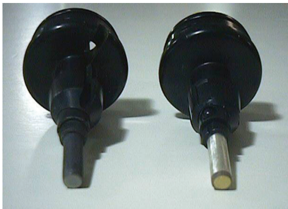
Figure 3. On the right is a properly prepared cathode and anode. Note the light silver appearance of the anode and matte finish of the gold cathode.
