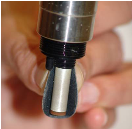
Figure 5. The silver cathode being sanded with a 400 grit wet/dry sanding disc to properly clean the anode from build-up and tarnishing.
