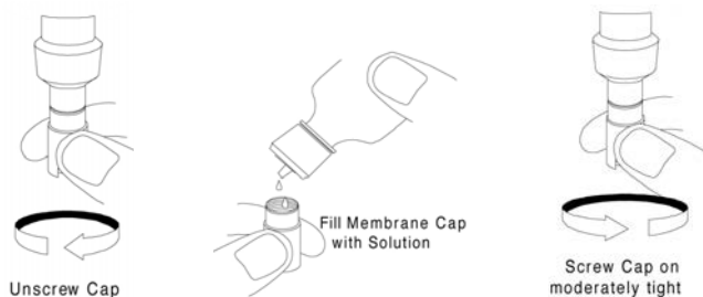
Figure 2. Installing a cap membrane couldn't be easier. Unscrew the old cap and discard. Fill the new cap a little less than halfway with solution. Screw the cap onto the sensor and rinse off any extra solution.
