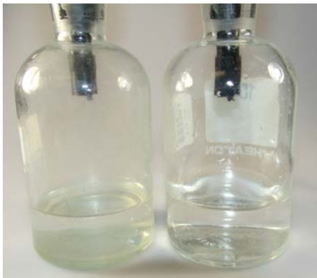
Figure 6. The calibration bottle on the right is clean. The calibration bottle on the left actually has algae growing in it which could affect the calibration values.
